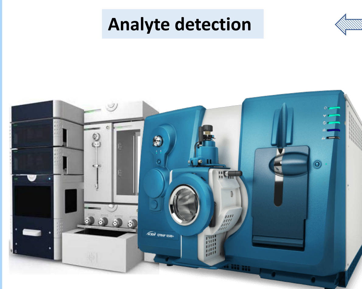
Fig 1. Analyte detection by LC-MS/MS Instrument Sciex Qtrap 6500 and spark Holland SPE/HPLC system.
