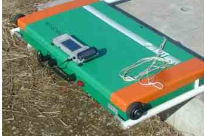
Figure A22. Properly positioned scan unit against the stopper for accurate determination of bar positions along the joint.
