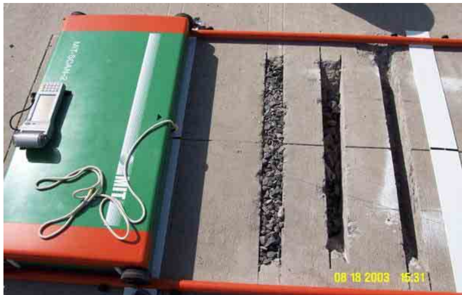
Figure 9. Dowel covered with aggregate for the evaluation of the effects of cover material.
