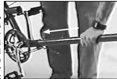
Fig. 7 Bottom tube installation.
