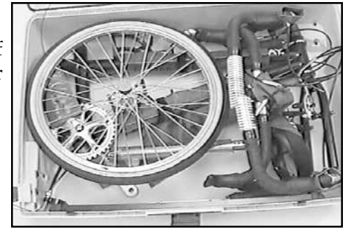
Fig. 27 Front wheel placement.
