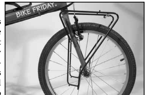
Fig. 6 Completed front rack.
