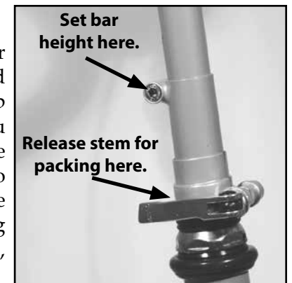
Fig. 26 Adjustable stem.
