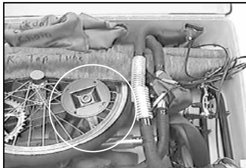
Fig. 31 Crush protector placement.
